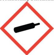
**SECTION 3: Composition/information on ingredients:** Compressed Gas: Air with up to 15% helium.
