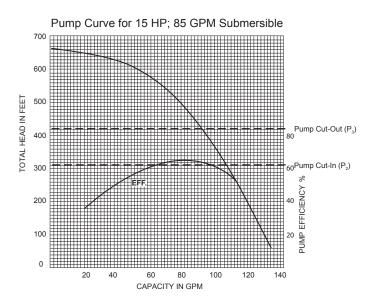
Subtracting the feet of head required for lift of 240' we can convert this point to PSIG:
