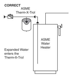
Let's explore the effect of placing the Therm-X-Trol on the hot water outlet. As thermal expansion takes place, heated water flows from the water heater outlet into the expansion tank. As water sits in the tank, it begins to cool. As previously explained, water is expelled from the tank during a demand. Since this water has cooled, hot water will not be immediately available at the fixtures.
