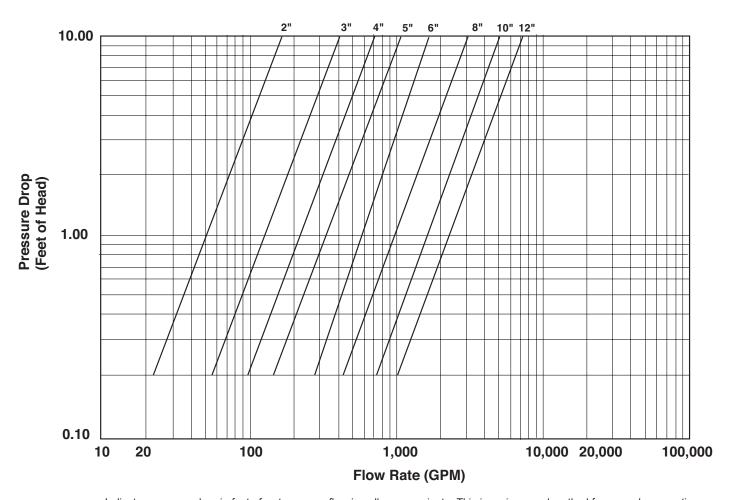
Indicates pressure drop in feet of water versus flow in gallons per minute. This is an improved method for properly computing pressure drop in AMTROL Separators.
